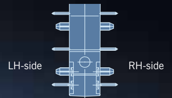
Side definition with terminals and location pins
